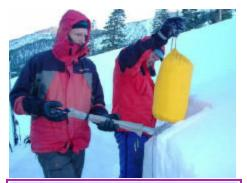
Pictured above and to the left are members of the Mono County Search and Rescue Team engaged in stuff block tests and snow crystal identification.
